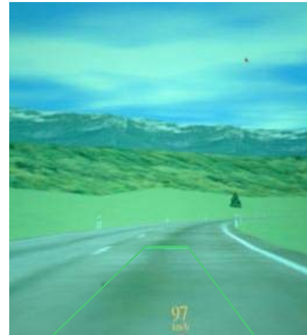
Breaking bar & drive-path
